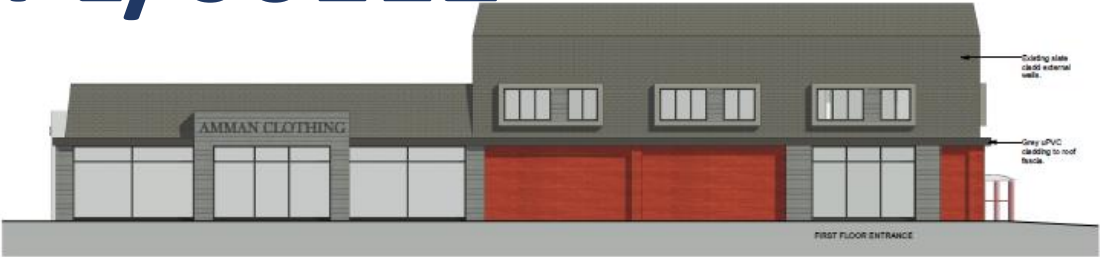
1 North East Elevation 1 : 100 0m 2m 4m 6m 8m 10m VISUAL SCALE 1:100
